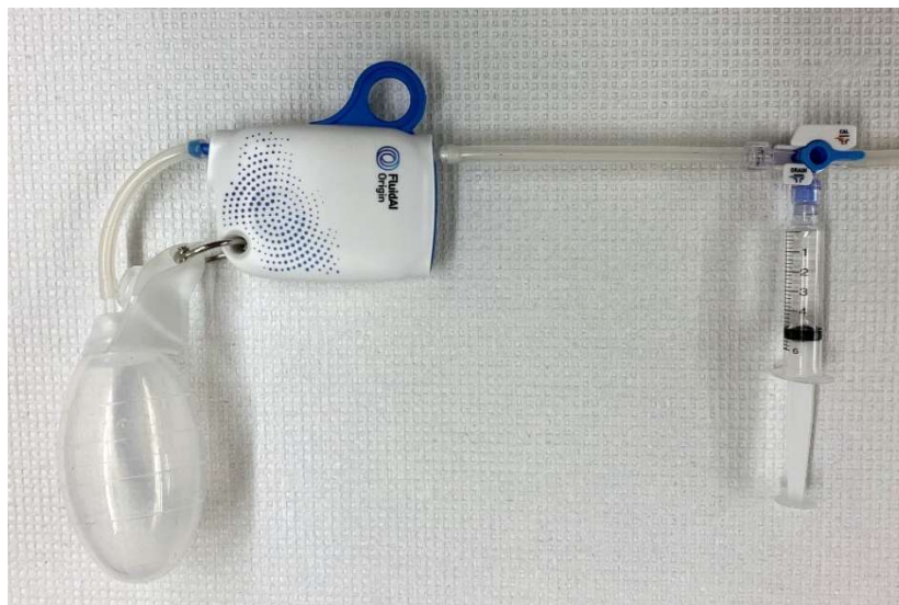
Figure 66: Origin ™ stopcock "OFF" towards the "CAL" or calibration mode
